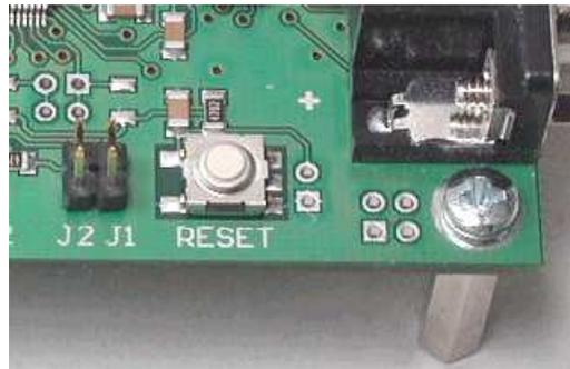
Pressing the reset switch causes a hardware reset of the microcontroller.
