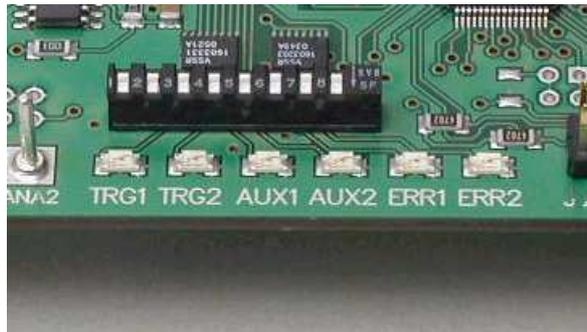
There is a display of six LEDs controlled by the microcontroller. TRG1, TRG2, AUX1 and AUX2 are yellow, and ERR1 and ERR2 are red. Please refer to the software section of this manual for the meaning of the LED signals.
