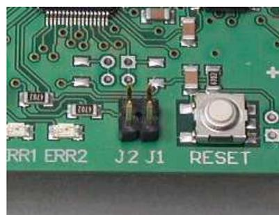
The headers J1 and J2 can be used for the same purpose as the SIL switch (see above) by installing jumpers or connecting external switches. They can also be used as I/O connections for various purposes. Please refer to the software section of this manual for more information.
