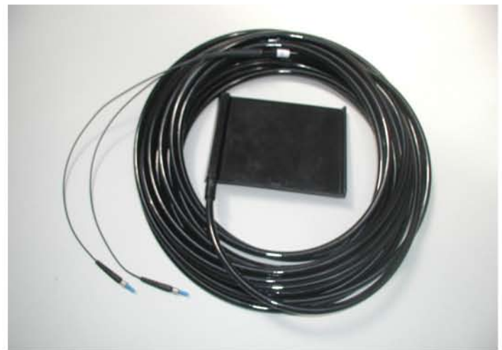
FORPS – Fiber Optic Rail Pad Sensor
