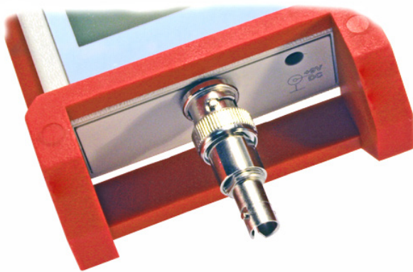
Pic. 3 BNC-socket with F-ST adapter
